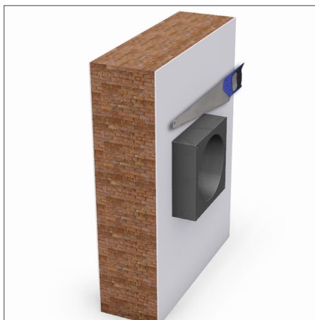
Fig. 4 – shortening the mounting block in a final step
